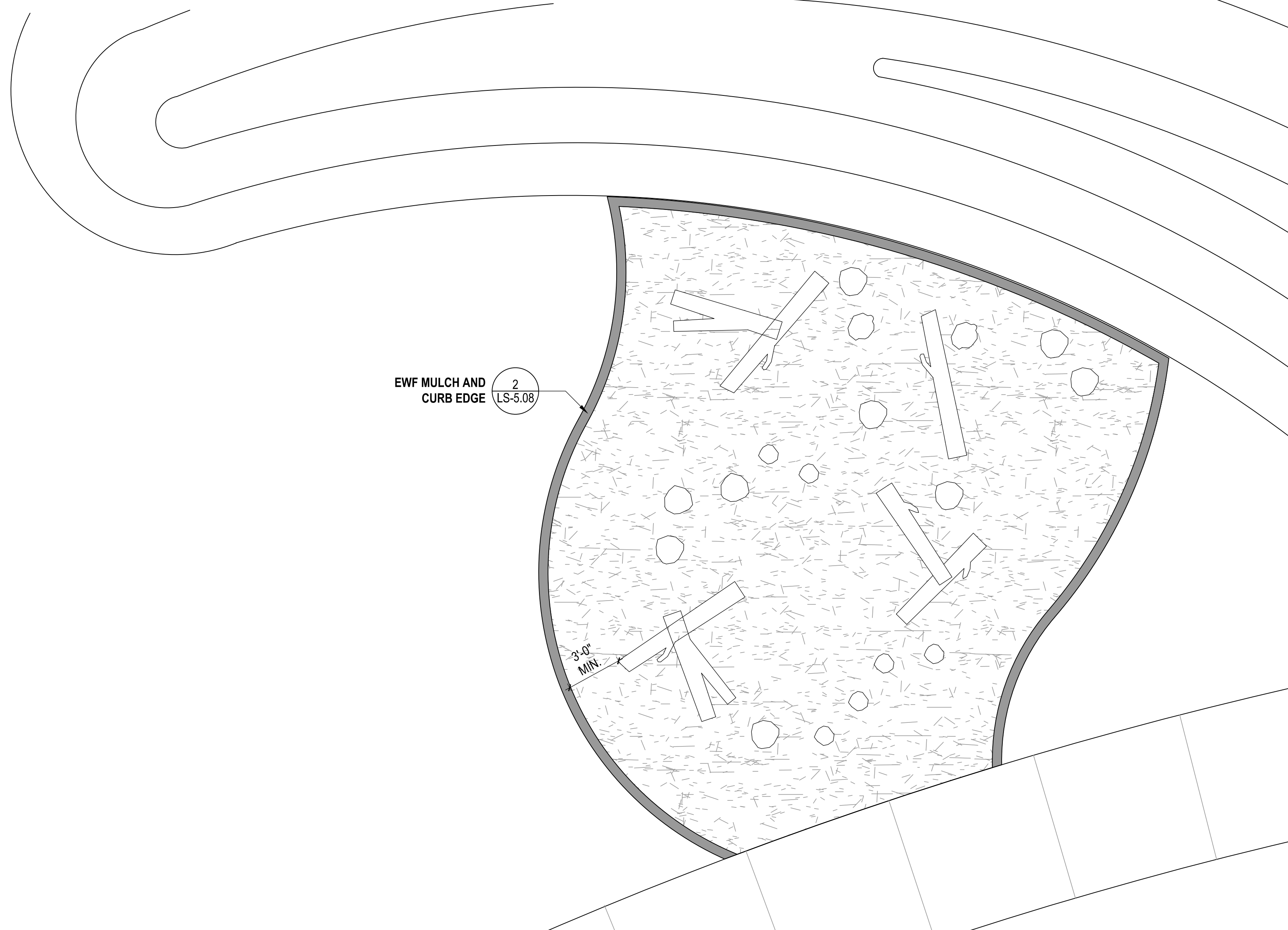
2 ENGINEERED WOOD FIBER MULCH AND CONCRETE CURB EDGE SCALE: 1 1/2"=1'-0" DT-EDGE CONC
